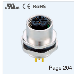
Gender: Female Coding: A, B, C, D Locking type: Fix screw (PCB) Mounting type: Rear fastened
