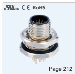
Gender: Male Coding: A, B, C, D Locking type: Fix screw (PCB) Mounting type: Front fastened
