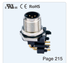
Gender: Male Coding: A, B, C, D Locking type: Fix screw (PCB) Mounting type: Right angled
