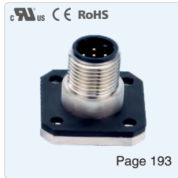
Gender: Male Coding: A, B, C, D Locking type: Fix screw (Solder) Mounting type: Flange
